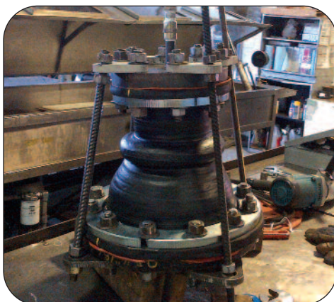
Thorburn's 42HP-CR Concentric reducer 300mm (12") by 125mm (5") ID tested at 16 bar
