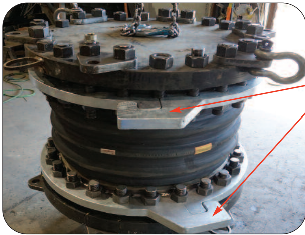
Style 301EF ultra high pressure 600mm (24") ID expansion joint being hydrostatically tested to 37 bar (540 psi)
